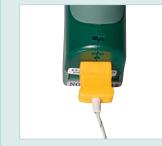
Type K input for contact measurements
